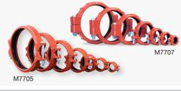
Made to USA standards, to easily interchange with other major manufacturers, the Munro standard and heavy-duty flexible couplings are ideal for use in countless piping applications where misalignment might be present. The M7705 and M7707 can accommodate vibration, thermal stress and moderate seismic activity. These tried and true couplings offer pressure capabilities to 750 PSI, depending on pipe size and wall thickness - choose the heavy-duty coupling for higher pressure requirements.
