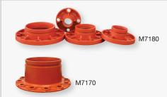
The flange adapter is the ideal product to transition from flanged to grooved components and is compatible with ANSI Class 125/150. Pressure ratings conform to the pressure rating of installed couplings. The all-in-one universal flange adapter accepts ANSI 125/150, PN10, PN16, JIS 10K and BS-10E flange patterns. In addition, a longer grooved-end makes this unique fitting easier to install.
