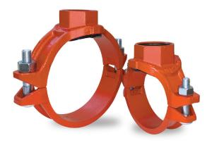
Mechanical tees, sometimes called a saddle tee, allow you to create a mid-pipe branch outlet quickly and easily. A gasket seals on the joined pipe, in the neck of the outlet. The connection is female threaded. These fittings are not recommended for vacuum applications.
