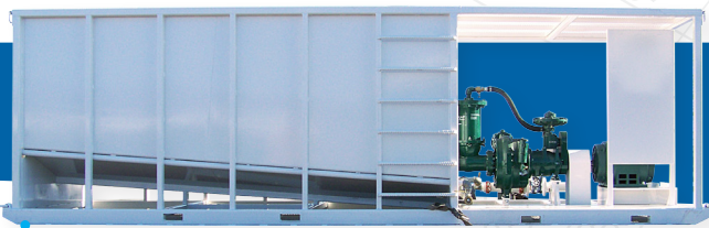
Dewatering with Fine Particulate Signal Peak Coal Mine Central Region, MT
